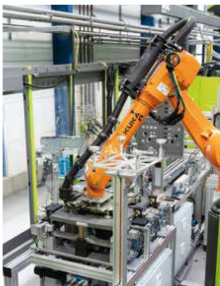
In the fully automatic pallet assembly, the robot presses the deck onto the three runners.
