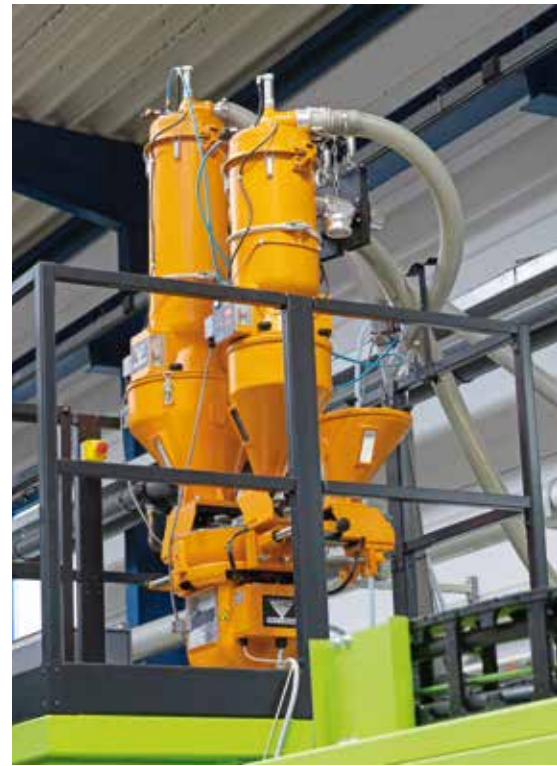
For the new pallet, as on all the machines, gravimetric metering of virgin material, recycle and masterbatch ensures the exact composition of the injection moulding compound.
