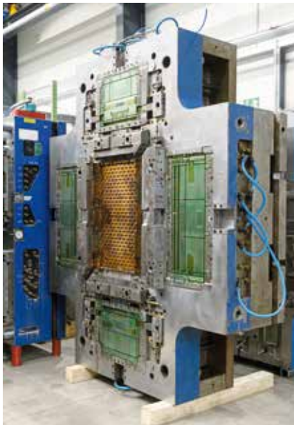
A typical injection mould for five of the eight elements of a folding box.
