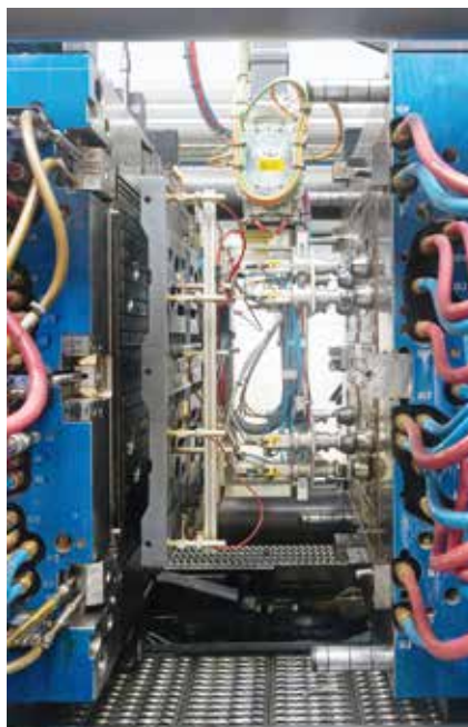
View into the injection mould for the pallet deck: the robot removes the finished deck on the left and places the TPE inserts for the next pallet on the right.
