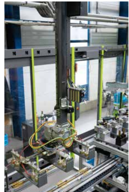
The three runners of the pallet come out of the second injection moulding machine.
