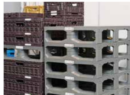
All modern load carriers are marked with labels or RFID tags via IML processes.
